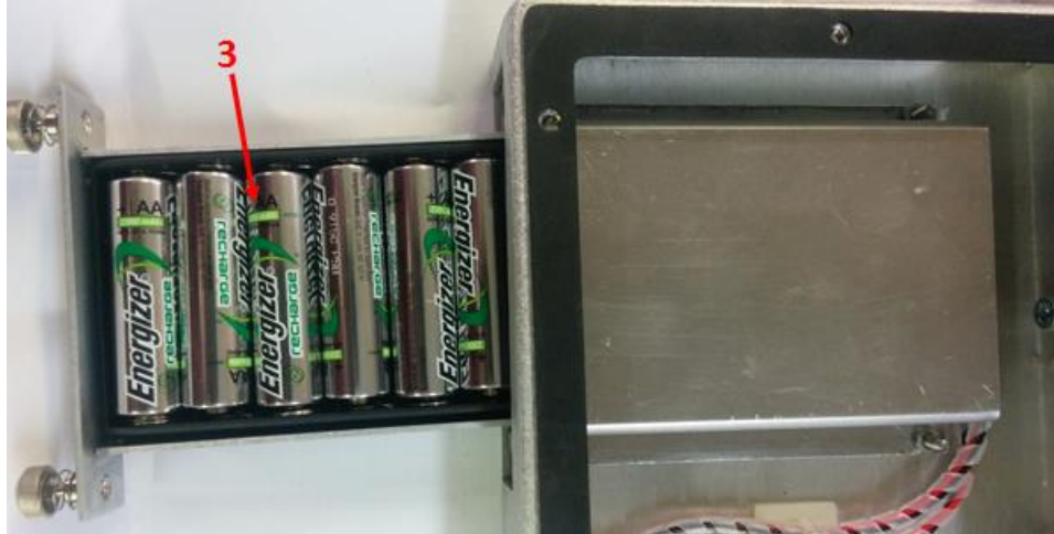
Figure 4-2 Platform Scale Battery Removal
